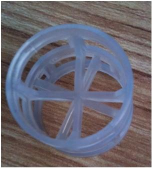
**FEP** means Fluorinated ethylene propylene, it is a copolymer of hexafluoropropylene and tetrafluoroethylene. We make **FEP pall rings**, it is different from PTFE pall rings, as **FEP pall rings** can be made by injection machines, but PTFE pall rings can only be made by moulded.
